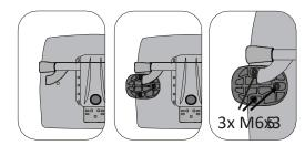
5. Place the seat on the pneumatic lift cone.
