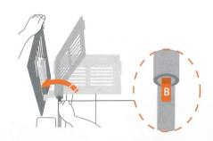
Press Button and rotate the support board upwards by 90°.
