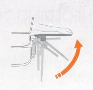
3 Turn up the support board by rotating it upwards to 90°.
